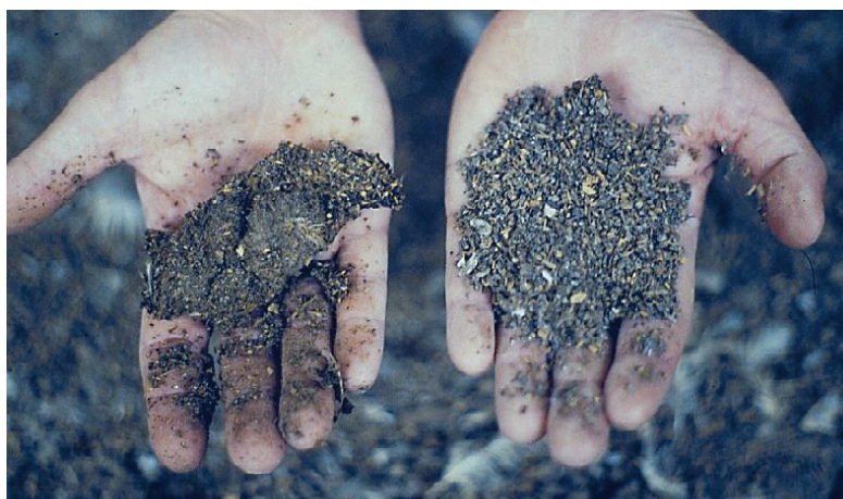
Left sample: too wet, not acceptable. Right sample: about right, acceptable.
